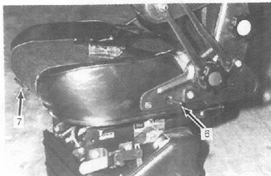
Figure 57: 4. Backrest Vertical Adj. Knob 6. Fore/Aft Adj. Handle Knob 5. Vertical Adj. Knob 7. Seat Tilt Adj. Handle Knob
