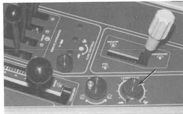
Figure 12: Lowering Rate Adjustment
